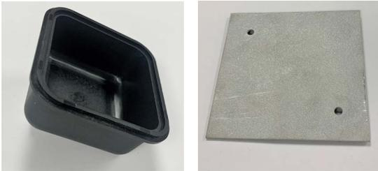
To test burst strength of the Zytel® Bonding Technology, the team injection molded a test cube that would represent a typical polyamide component (left). An aluminum plate was pre-treated to remove aluminum oxide (right), then Zytel® Bonding Technology was applied.
