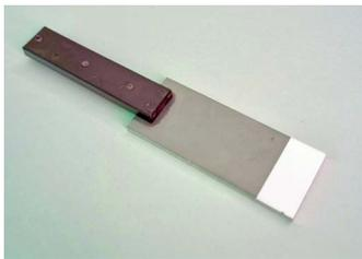
Lap shear strength tests were performed using Zytel® Bonding Technology and a conventional adhesive. Depending on the material tested, bonded samples had anywhere from 2x to 8x higher shear strength.
