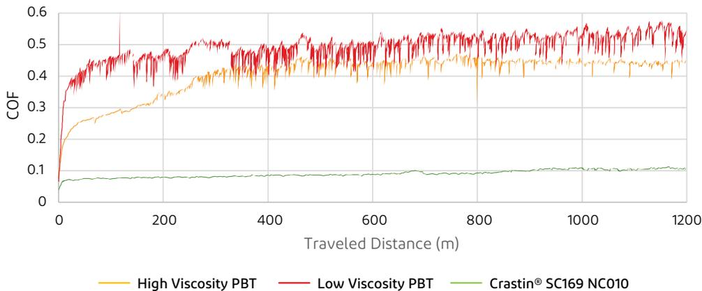
Internal test method against steel ball. Source: DuPont
